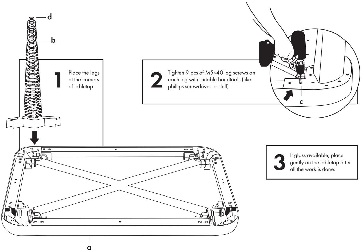
! Please be sure not to miss any screw holes and fasten all screws equally and tightly. Otherwise, you may face breakage or cracking during the time of usage.
